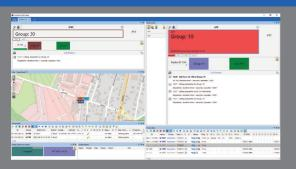
View of the dispatcher console working with two wide-area systems (IP Site Connect and Capacity Plus Multi Site). LOCATION POSITIONING module running. The console shows the use of the function key functionality (direct call to an individual contact or a group).
